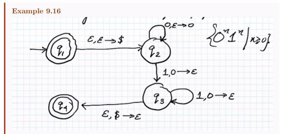
You are required to go all the way to the end of the input or you are jammed and rejected. This is an example of a deterministic machine but in general you can have non determinism.
