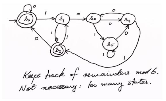
$\delta(s_0, 0) = s_0 = \delta(s_3, 0)\delta(s_1, 1) = s_1 = \delta(s_3, 1)$
