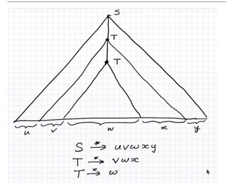
It is not possible that both v and x are empty. This is true if we assume Noam Chomsky form. But then we can change the second T into generating vwx which would mean thta  $uv^2wx^2y \in L$ . And you can do this again which would mean  $uv^3wx^3y \in L$ . We conclude that
