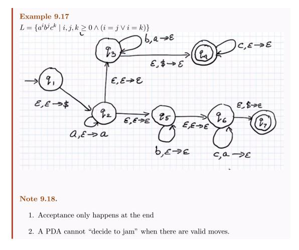
Note 9.19. There is an alternative notion of acceptance: no accept states, we accept if the stack is empty at the end of the input. These are equivalent.
